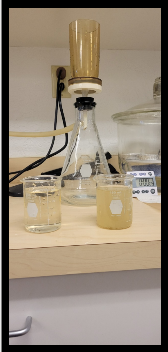
Sample at the Aspen Wastewater Treatment plant (Effluent Left, Influent right)
